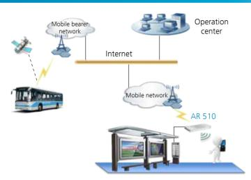
The AR510 can be deployed in a bus station to build an intelligent digital platform. The bus station using the AR510improves the functions of a traditional bus station because now it candeliver accurate schedule information by time and position. Passengers can find out about bus arrival times and distances in real-time.
