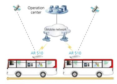
The AR510 can be deployed in a bus to provide a mobile interconnection solution. As the mobile gateway, the AR510 supports LTE/3G, and provides free Wi-Fi access so that users can enjoy Internet surfing anytime.
